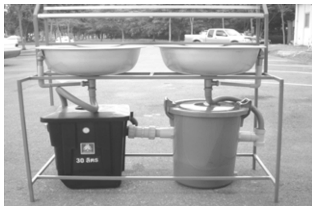
Figure 1. Low-cost wastewater treatment unit placed underneath dishwashing basins for floating food vendors.
