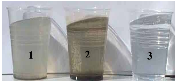
Figure 5. ECR Treated water (1: Before ECR, 2: Settlement after ECR, 3: After Filtration).
